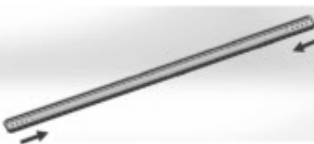
Drawing 15: TOP ALUMINUM STIFFENER WITH LEVEL RAIL MOUNTING BRACKETS
