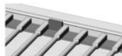
Drawings 4B & 4C: PRE-DRILL 1/8” DIAMETER HOLES THROUGH PVC RAIL & INTO BALUSTER INSERT & SCREW RAIL TO BALUSTER INSERTS
