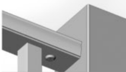
Drawing 21: RAIL ASSEMBLY PRIOR TO DECORATIVE TOP RAIL INSTALLATION
