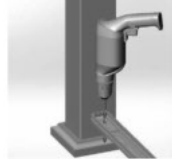
Drawing 10: DRILL ATTACHMENT BRACKET MOUNTING-BOLT HOLE THROUGH ALUMINUM STIFFENER
