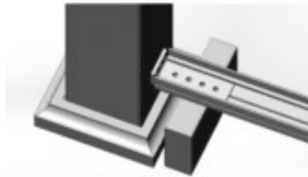
Drawing 7: ALUMINUM STIFFENER RESTING ON 2X4 BLOCK
